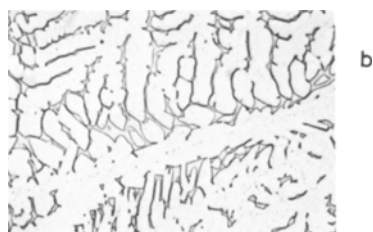
Fig. 10 (a) D_M curve for Cu-8%Al alloy. (b) Microstructure of this alloy, 110X.
