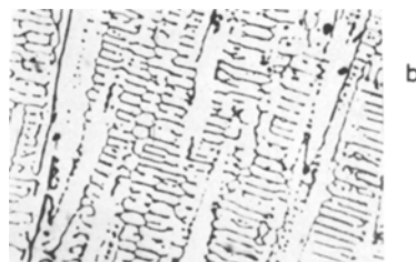
Fig. 2. (a) D_M curve for Cu-1%Zr alloy. (b) Microstructure of this alloy, 110X.
